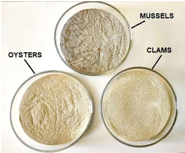
Figure 1. Sea shell powders (granulometry between 60 and 250 microns)
