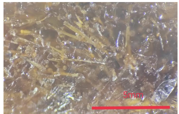
Figure 5. Posidonia fibers distribution in a relevant sample
